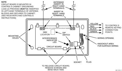
Figure 9. 5881/5882 RF Receiver (cover removed)
